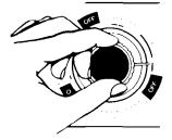
Set the washer for a DRAIN and SPIN (see page 8). Let it run for about 30 seconds to mix the antifreeze and water.
